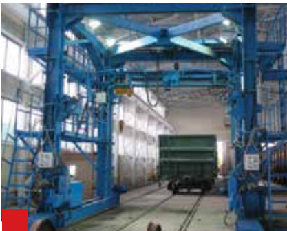
Specialized wagon – repair system WRS «Vityaz». The customer – «Russian Railways» Inc.
