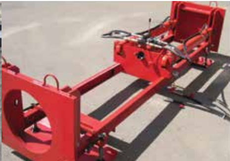
Equipment of a ground puncture – 25U UPG «Arrow» for trenchless installation of underground utilities. Manufacturing and supplying it to companies specializing in the laying of utilities.
