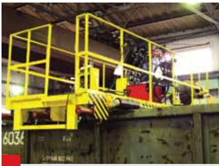
Installation for straightening upper capping frame of gondola wagons UP–2M to «Russian Railways» Inc.
